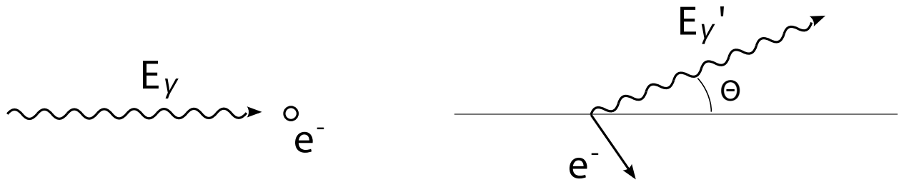
Figure 4.11 Schematic illustration of Compton scattering. Picture taken and modified from [3].
